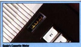
Trying to set a cassette recorder to the right volume level for the computer can be extremely difficult, but the Colour Genie has its own tape meter to make writing to and reading from a cassette considerably easier
