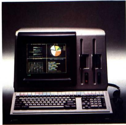
internal functions, such as checking the keyboard and controlling the screen. One method is 'interrupt-driven' where a special electronic circuit interrupts the microprocessor perhaps 50 times every second and 'reminds' it to perform its housekeeping tasks and other functions on the screen and keyboard, before resuming what it was
