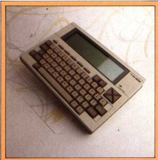
NEC PC8201A Although the NEC PC8201A is exactly the same size as its siblings, this machine has a significantly different keyboard. The cursor keys have been moved out into a small cluster, the function keys have been reduced from 8 to 5, and the keyboard layout is slightly different. In addition, the NEC has only three of the standard programs in ROM: Text, Schedule and Telecom
