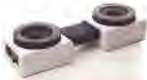
Protok 1200 Type: Acoustic modem Baud Rate: 1200/75 and 1200/1200 Price: £89.95
