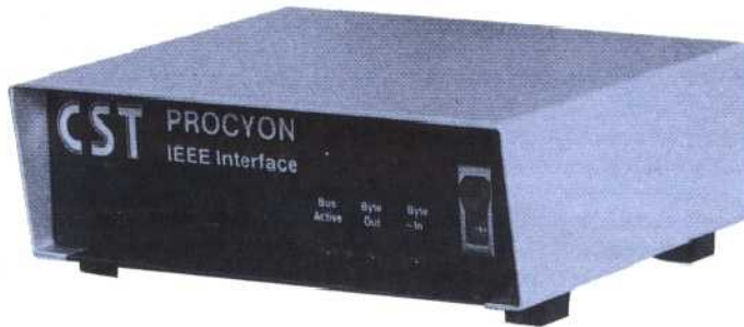
An IEEE-488 interface, designed for use with the BBC Microcomputer.
