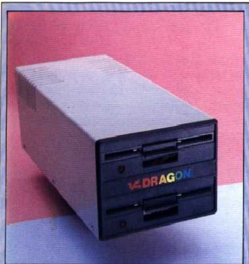
Dragon Disk Dragon's disk unit has either one or two drives of 175K each. The unit comes with the small but adequate Dragon DOS built into its interface cartridge
