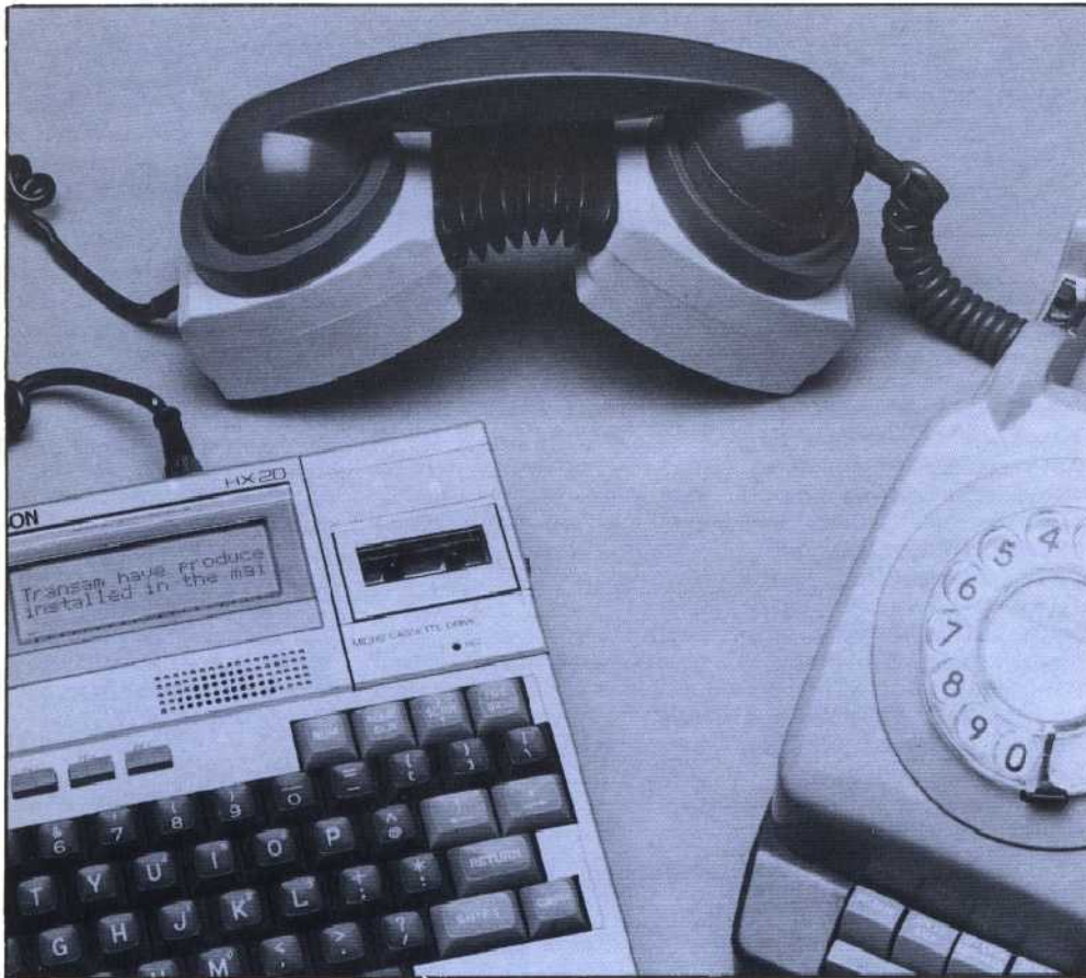
An acoustic coupler like this links a computer to the telephone network.
